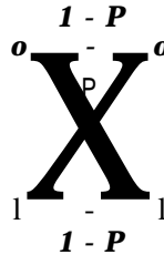
Figure 2.8 A binary symmetric channel. A 1 or a 0 in the input gets flipped on transmission with probability p .
